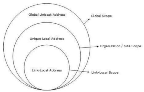
[Image: IPv6 Unicast Address Scope]
